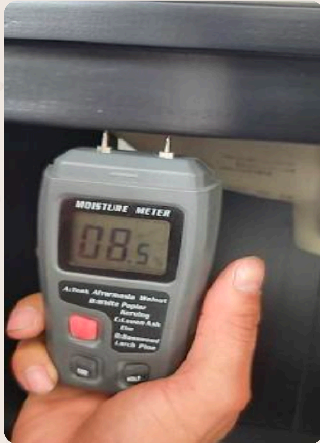
Moisture content inspection
